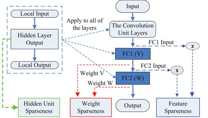
**Fig. 3.** The hidden unit, weight and the proposed feature sparseness.  $V$  and  $W$  are the weight matrices linking the FC layer input with the corresponding output.  $z$  and  $x$  are the inputs of FC1 and FC2, respectively.
