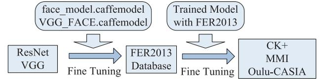
Fig. 5. The fine tuning of models for different databases, i.e. FER2013, CK+, Oulu-CASIA and MMI. face\_model.caffemodel and VGG\_FACE.caffemodel are two CAFFE model trained for face recognition corresponding to networks ResNet and VGG, respectively.
